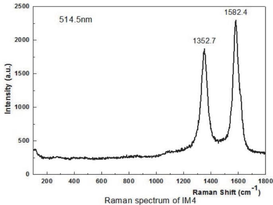
**Figure 8.** Raman spectrum of industrial type MWCNTs.
