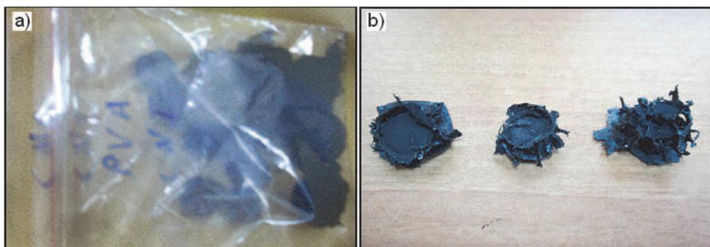
**Figure 4.** Preform samples (a) packed for usage after curing and (b) before curing.
