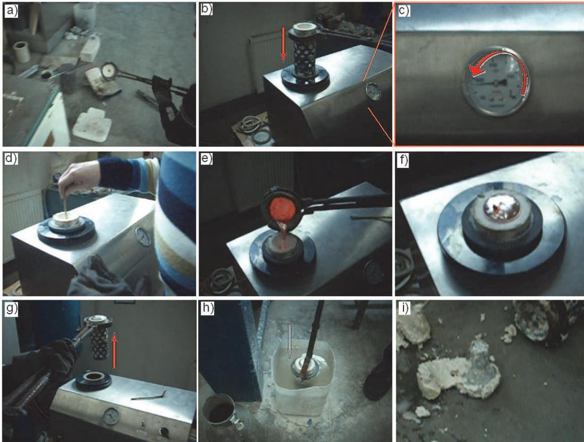
**Figure 6.** Vacuum assisted infiltration process steps: (a) Flask taken from furnace, (b) locating the flask, (c) vacuum pumping, (d) placing the preform, (e) pouring the molten metal, (f) solidification under vacuum, (g) removing flask for solidification in the air without vacuum, (h) sinking flask into the water and (i) cast composite with runner.
