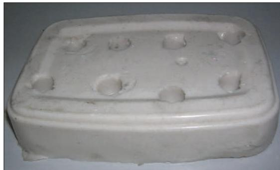
**Figure 3.** Flexible preform mold.
