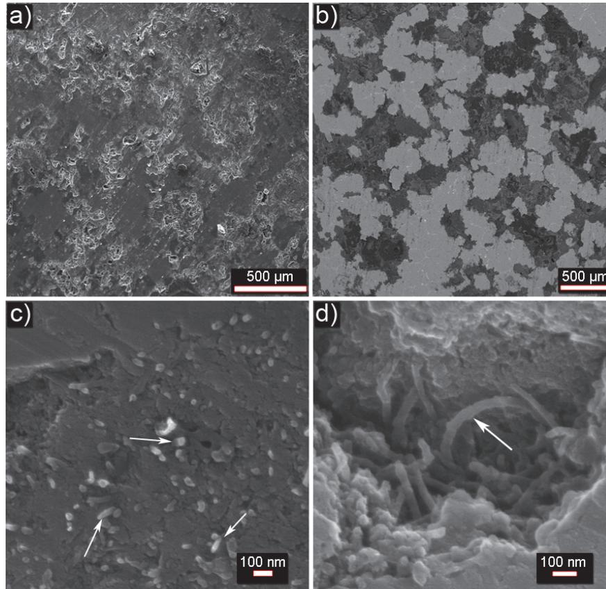
**Figure 9.** Distributions of Al and CNTs in composite were shown by: (a, b) SEM images of polished composite surfaces and SEM images of the fractured and polished surfaces of composites, (c) showing the pulling-out of CNTs between fractured surfaces and (d) showing the bridging of CNTs between different sides of matrix material.
