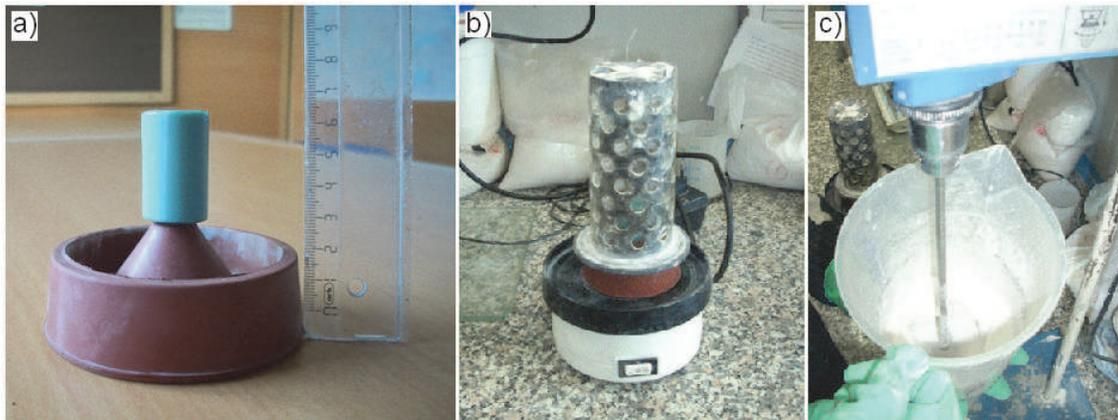
**Figure 5.** Materials and devices used for mold preparation:(a) wax pattern mounted to the runner head, (b) flask on the vibration machine and (c) preparation of gypsum slurry with mechanical mixer.
