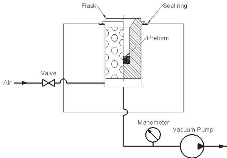
**Figure 7.** The schematic diagram of vacuum assisted infiltration system.
