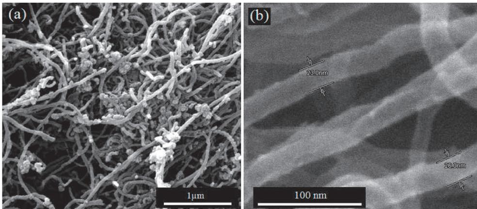
**Figure 2.** Electron microscope images of CNTs: (a) Secondary electron SEM micrograph of industrial type MWCNT's and (b) TEM micrograph showing the average diameter of MWCNTs is between 10-30 nm.
