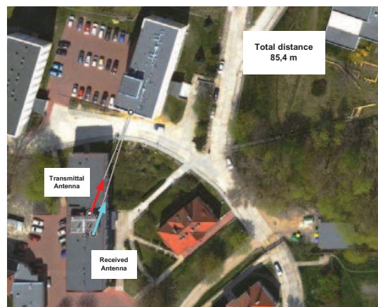
Figure 4. Approximate determination of second path of signal propagation from transmitting to receiving antenna
