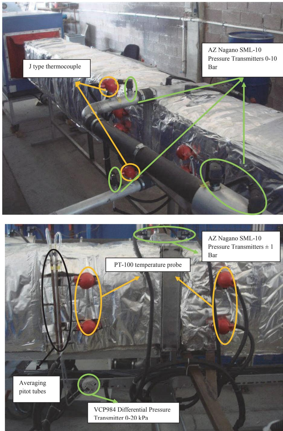
**Figure 6.** Measurement points in the experimental setup.
