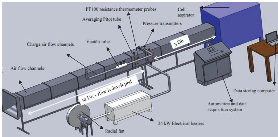
**Figure 1.** 3D solid model of experimental setup for intercooler tests.
