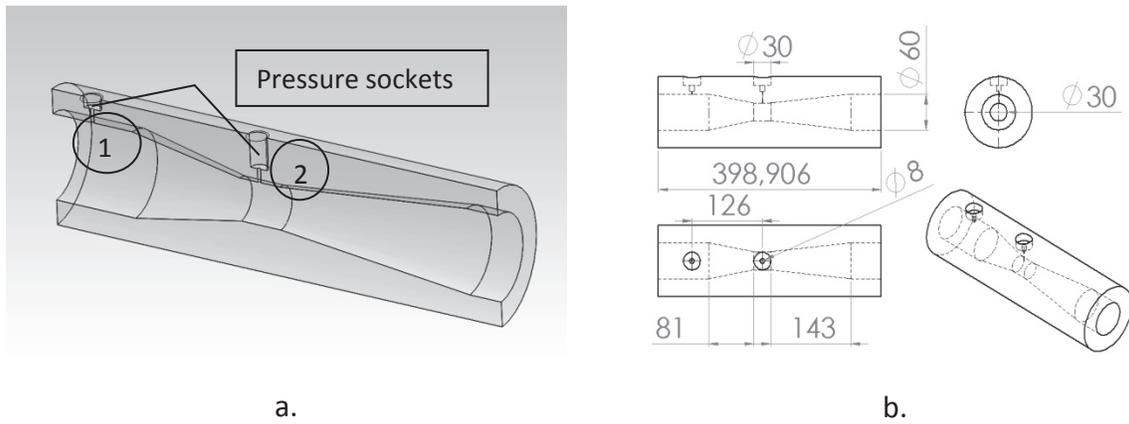
Figure 3. A-Cross section of venturimeter, B-Venturimeter for hot gas channel.
