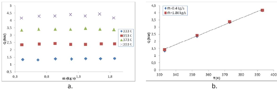
Figure 11. A-Intercooler cooling capacity a. at four different charge air entrance temperatures changing with mass flow rate of cooling air, B-at maximum and minimum mass flow rates of cooling air changing with temperature.
