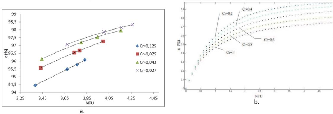
Figure 9. A-Intercooler ε-NTU,B-Calculated ε-NTU.
