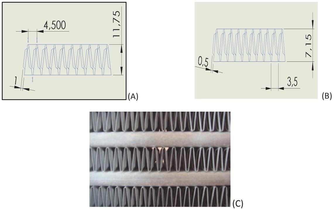
**Figure 7.** A- Fins in cooling air passage, B- Fins in charge air passage, C- Louvered fins.
