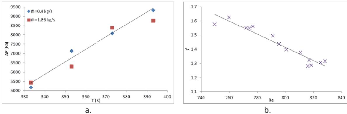
Figure 12. A- Pressure drop in intercooler changing with mass flow rate of cooling air, B-Friction coefficient changing with charge air Re numbers.
