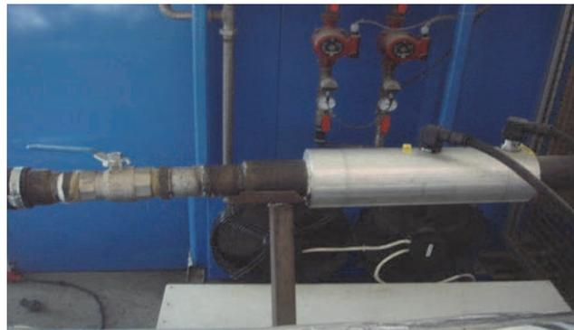
Figure 4. Venturimeter for hot gas channel.
