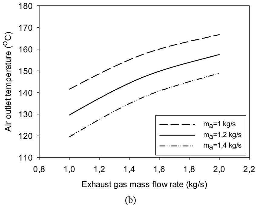
**Figure 4.** The variation of outlet temperatures for  $T_{g,i}=200^{\circ}\text{C}$ ,  $T_{a,i}=25^{\circ}\text{C}$  a) exhaust gas b) air
