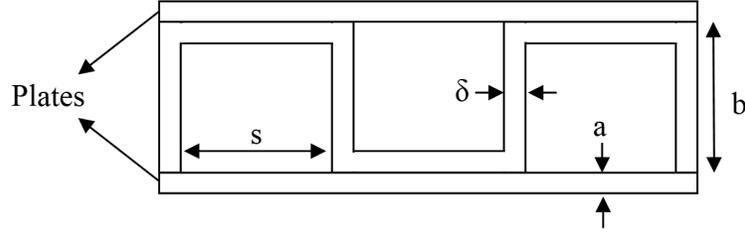
Figure 2. Schematic representation the dimensions of offset strip fin [1]
