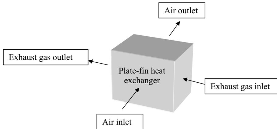
Figure 1. Schematic representation of plate-fin heat exchanger
