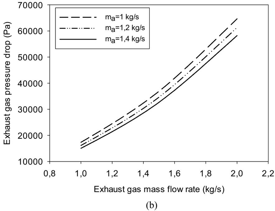
**Figure 6.** The variation of exhaust gas pressure drop with mass flow rate
